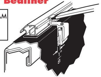
For each clamp mark on your bedliner a 1-1/2" x 3" hole as shown above. Remove clamp. Cut holes in bedliner. Reinsert side rail clamp. Return to step 5.
