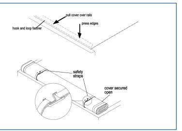
8. Your Tonno Pro Low Roll cover has been set at the factory for moderate tension to keep your cover free of wrinkles. Dependent on weather conditions it may be necessary for you to adjust the tension control on your cover. To adjust your tension control, simply loosen the fasteners on the front bulkhead and lift up the bulkhead. Once the bulkhead is loose, simply slide the tension control plate towards the cab of the truck.
