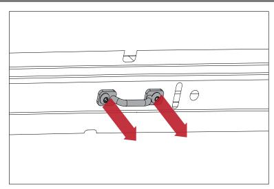
2. Reuse factory Torx Screws to install CB Mount with footman loop on outside as shown.
