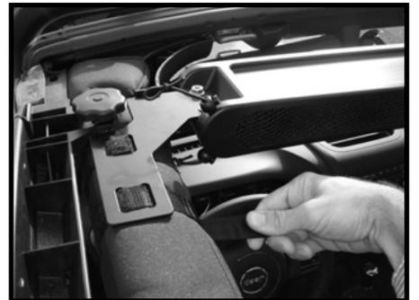
3. Insert the Short Velcro Strap through the slot in the rear of the Storage Console and attach to the footman loop of the windshield.
