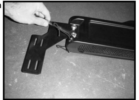
2. Place the Storage Console inside the vehicle such that the mounting brackets rest on the roll bar. The Storage Console should sit just above the visors. Insert Long Velcro Straps through the slots in each Mounting Bracket and strap them tightly around the roll bar on both sides of the vehicle.
