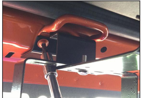
6. For 2011+ JK's: use factory Torx screws to install CB Mount and footman loop with CB Mount on outside.
