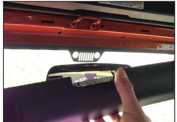
2. For 2007-2010 model JK's: drill out rivets using 3/8" drill bit. Rivets will be replaced with Well Nuts.
