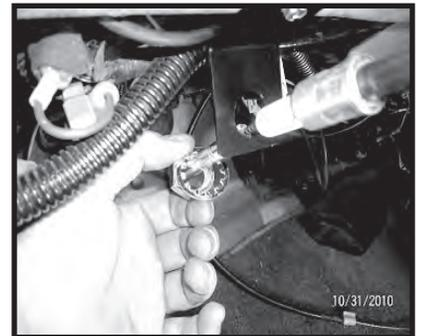
**Step 3.** Remove the factory actuator housing. Unplug the factory wiring clip from the sensor on the actuator housing (If Equipped). Remove the vacuum lines from the vacuum diaphragm. Before you unbolt the actuator housing, place a drain pan under the axle to catch any fluid that may drain out. With the actuator housing removed, all gasket material and dirt or debris will need to be cleaned and from the surface and inside the housing. The diaphragm shield may be removed if needed.
