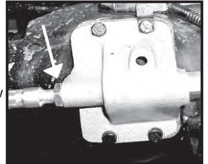
Step 7. Install the vent hose in the new housing (If Equipped). If the factory cover did not have a vent hose, install the supplied plug. Install the four wheel drive indicator switch into the new housing, thread locker will be needed. Refill the differential if any fluid was lost.
