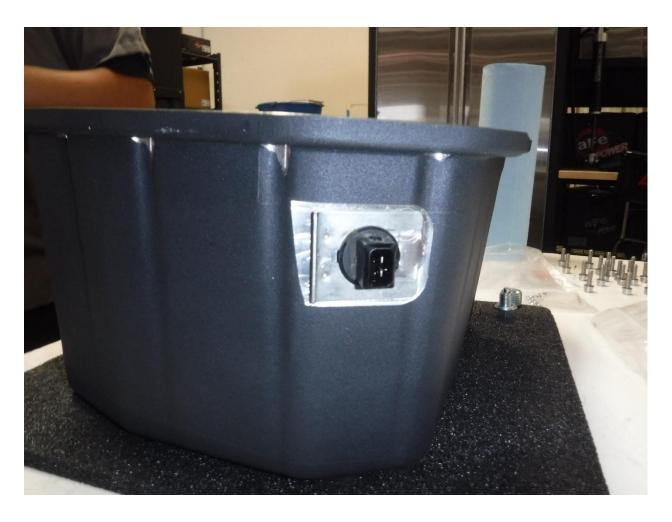
18. Carefully install the sensor connector in the aFe oil pan by pushing it through from the inside of the pan.
