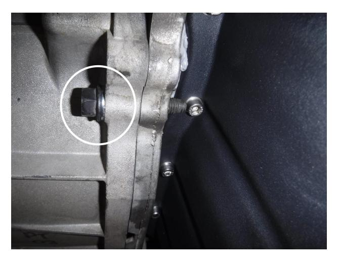
30.Re-install the transmission bolt removed in step 11, using the supplied M10 flat washer.
