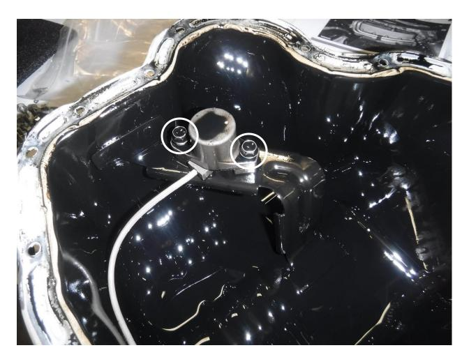
15. Remove the two (2) screws holding the sensor to the bracket inside the oil pan.
