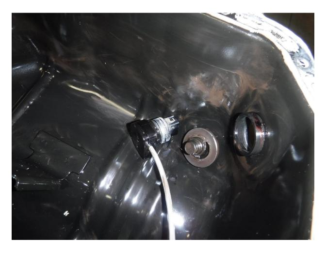
14.Once this holding clip is removed, push the connector towards the inside of the pan.
