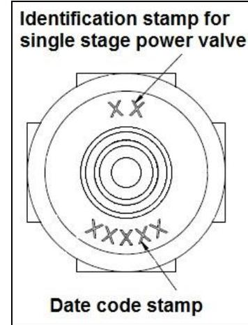
Example: If your current power valve is stamped 12, Holley suggests replacing it with a power valve stamped 65.
