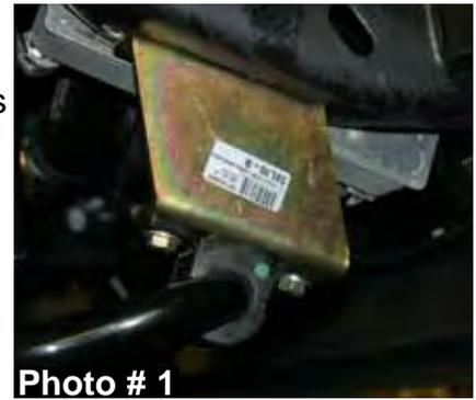
5. Attach the OEM sway bar to the new Skyjacker sway bar lowering brackets using the supplied 7/16" x 1 1/2" fine thread bolts, washers, & nuts. (See Photo # 1) **Note:** Fully tighten all hardware at this time.
