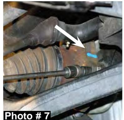
10. Remove the OEM upper & lower a-arm ball joints from the OEM steering knuckle using a 18mm & 24mm socket. It may be necessary to strike the steering knuckle to allow the ball joints to dislodge. **Note:** Be careful not to damage the ball joints. Remove the OEM steering knuckle from the vehicle.
