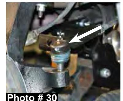
Passenger side shown with one 15/16" cv-spacer.
