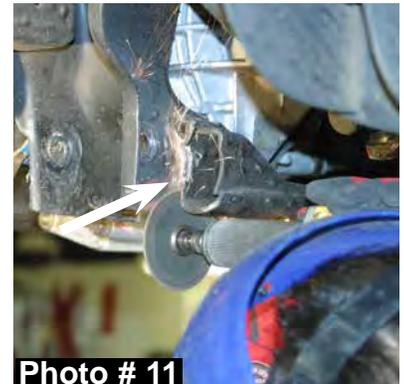
15. With the welds ground off, remove the cross member mounting bolts using a 18mm wrench & remove the rear cross member assembly. (See Photo # 12)
