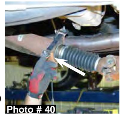
45. Once the nuts are removed, knock out the OEM studs & install the new Skyjacker carrier bearing lowering spacer using the supplied 3/8" x 3 1/2" fine thread bolts, washers, & nuts. **Note:** Install the new carrier bearing lowering spacer using the 2" side. (See Photo # 41)
