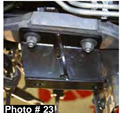
25. Remove the OEM bump stops from the frame using a 15mm socket. Enlarge the two OEM bump stop bracket bolt holes, using a 7/16" drill bit. Install the new Skyjacker bump stop bracket using the supplied 7/16" x 1 1/2" fine thread bolts, washers, & nuts. Center punch the remaining hole & drill using a 7/16" drill bit. Install the remaining 7/16" x 1 1/2" fine thread bolt, washers, & nut. (See Photo # 25)
