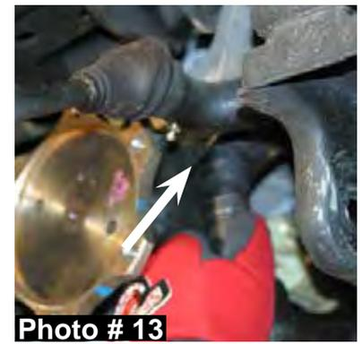
17. Remove the driver side upper differential bolt using a 21mm socket. Disconnect the vacuum hose on the driver side of the front differential & remove the differential using a transmission jack. (See Photo # 14)
