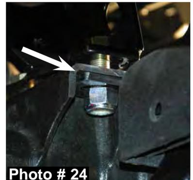
28. Attach the rear of the differential to the new rear cross member using the OEM hardware. Push the differential back toward the rear of the vehicle & tighten the bolts. Reattach the OEM front vacuum line & front actuator line.
