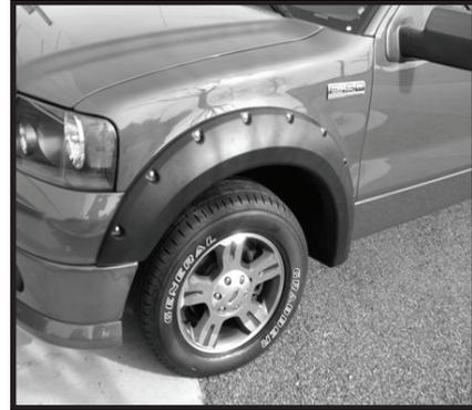
1. Install the supplied trim hardware onto the flares. Place a washer on the bolt and insert the bolt through the hole in the flare. Place a lock nut on the back side of the flare to secure the bolt.
