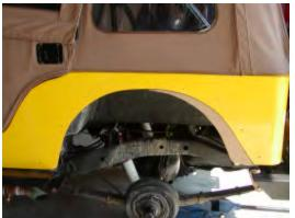
Some kits may include a pre-made template that will make the process quicker and easier. Simply install the template, trace, and make the cut.
