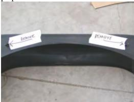
It is necessary to remove the two (2) locating studs from the rear flares. The studs are only used on TJs, and are not
