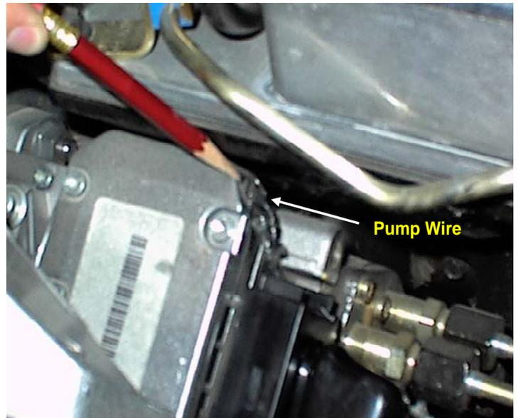
12. **NOTE:** Important-while the connector halves are being seated together the wire is not to be rotated. The stock wiring harness that plugs into the injection pump may be removed for better access to the wire. Connect the supplied gray wire to the supplied pin connector wire.
