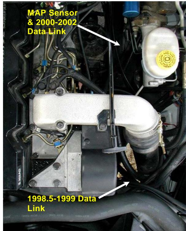
15. A plug is installed in the data link connector on the truck to resist corrosion, remove this and install the supplied connector.
