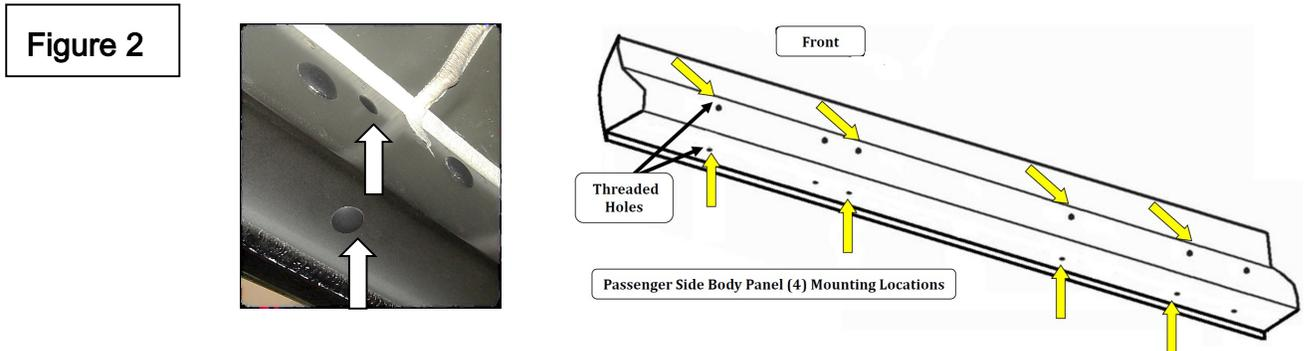
2. Install one of the brackets by positioning the bracket and attach to the rocker panel using (2) M8 x 25mm hex bolts, (2) 5/16" flat washers, (2) 5/16" lock washers. Leave the nuts loose for final adjustment, (FIGURE 3).
