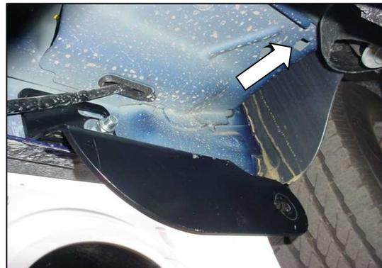
Insert into the square hole steel bar with 5/16" bolt.
