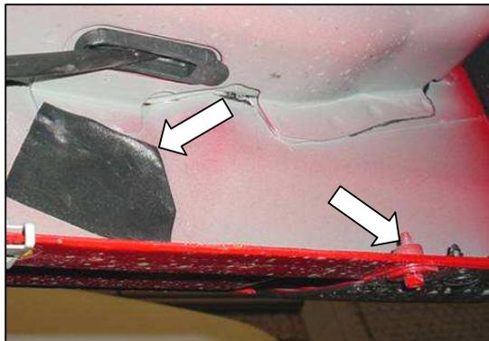
Remove this cover hole tape and bolt & clip nut.
